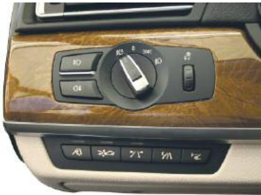
Light switch in position A
